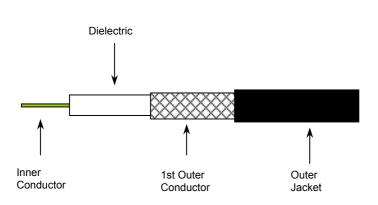
Series 58 Coaxial Cable Stranded Tin Copper Conductor Solid Polyethylene Dielectric 95% Tin Copper Braid Screen PVC Jacket
